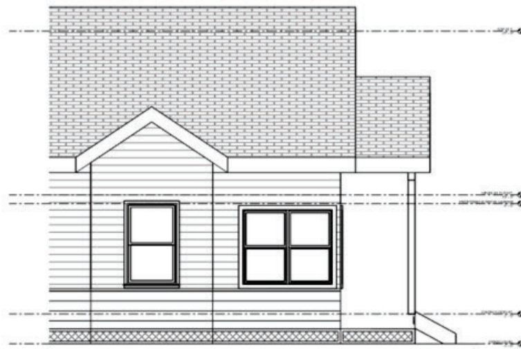
02 EXTERIOR ELEVATION - EXISTING SOUTH SCALE: 3/8" = 1'-0"
