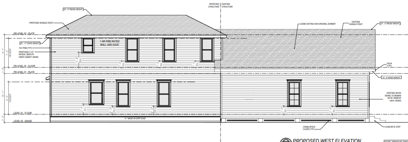
PROPOSED WEST ELEVATION Scale: 1/4" = 1'-0"
